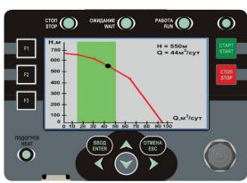
Adjustable graphic presentation of parameters on the drive's display or a PC
